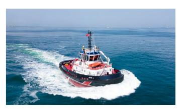
Built entirely from welded mild steel with twin rudders, the vessel ensures safe and efficient performance in various maritime tasks, including ship assistance, escort duties, external firefighting, and oil pollution control operations. The first VSP tugboat produced was delivered to Tripmare in Italy for service.
