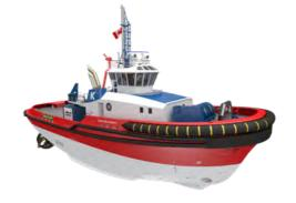
the most powerful escort tugs in Canada, capable of achieving a massive 120 tonnes of bollard pull, while also providing significant environmental benefits, reducing greenhouse gas emissions and underwater radiated noise.
